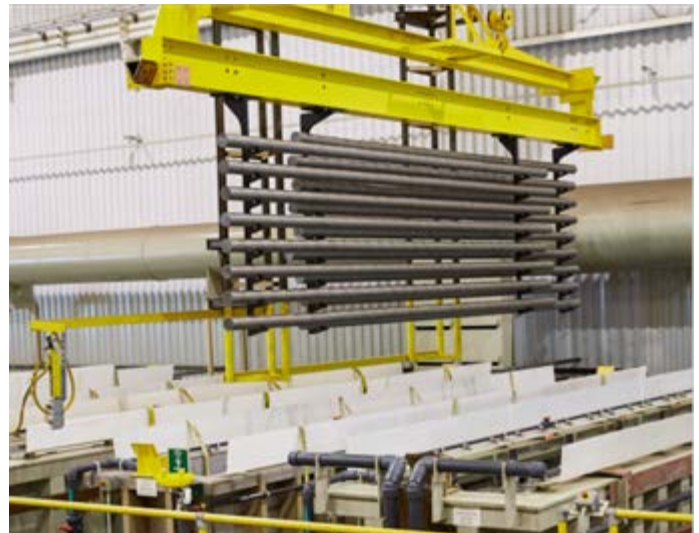
Figure 10 Bar Rack Supporting 17 up to 150 mm x 150 mm x 7.6 m (6" x 6" x 25') bars
