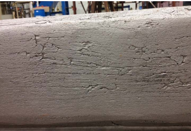
Figure 4. As-Forged and Blasted, 23 cm across the flats (9 inch) RCS Ti-6Al-4V Bloom Requiring Conditioning Prior to Subsequent Forging (Source: MetCon)
