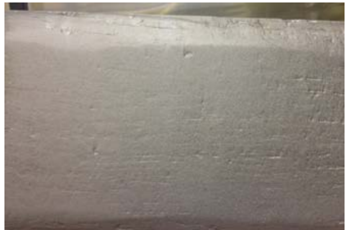
Figure 5. MetCon Electrochemically Conditioned 23 cm (9 inch) RCS Ti-6Al-4V Billet Conditioned to 2.3% Target Removal or 97.6% Step Yield (Source: MetCon)
