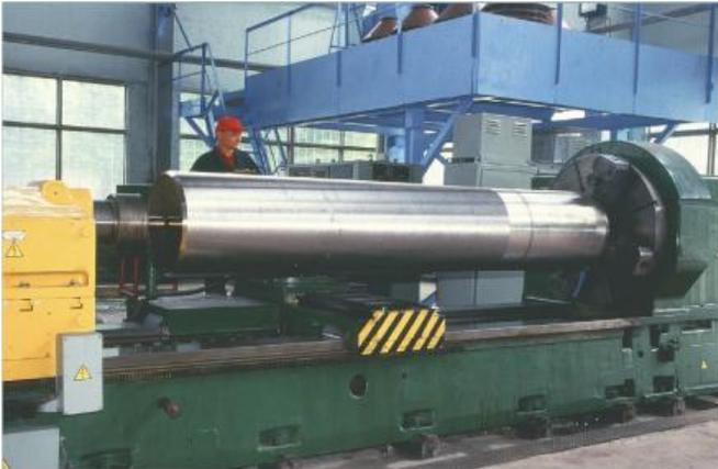
Figure 1. Lathe Turning Titanium Ingot (source: Antares)
