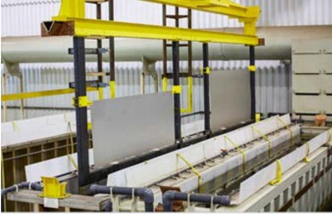
Figure 12. Sheet/Plate Rack Supporting up to One (1) 10 cm x 152 cm x 660 cm (4" x 60" x 260") or up to Two (2) 10 cm x 15 2cm x sum to 635 cm (4" x 60" x sum to 250") Sheets or Plates
