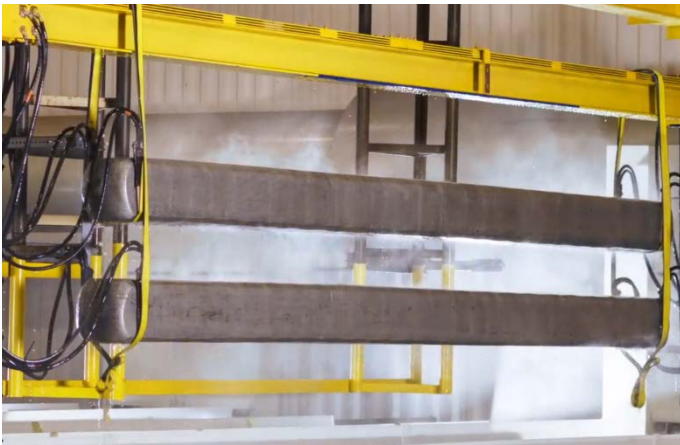
Figure 11. Lifting Straps Able to Accommodate Any Product Up To 81 cm x 167 cm x 66 0cm (32" x 66" x 260") and Less Than 8100kg (8 ton)
