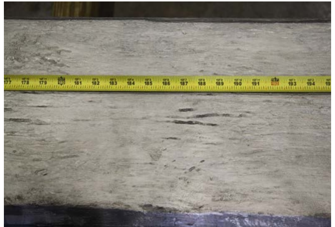
Figure 6. MetCon Black Markers of Remnant Alpha Case
